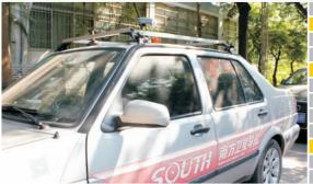
With the dimension of  $10\text{cm} \times 10\text{cm} \times 3.5\text{cm}$ , very lightweight, compact and rugged design, S650 and S660 are the most cost-effective gnss receiver. In this box, equipped with dual mode for Bluetooth V2.1 and Bluetooth V4.0, ensure the unit communicates cable-free with Bluetooth to your PDA terminal. What's more, this unit is able to work as an on-board equipment, greatly improve the working efficiency and the flexibility.
